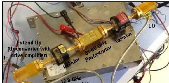
Fig. 17 – W-band (92 – 96 GHz) linearizer in test
