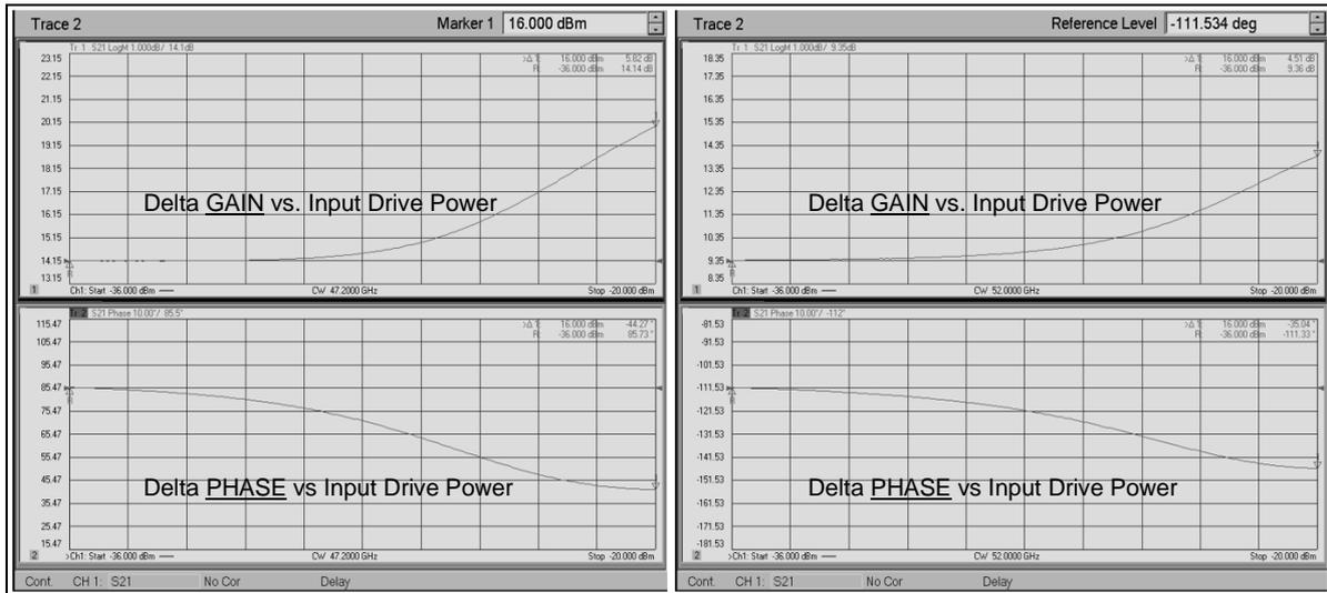
**Figure 12.** Linearizer transfer response (AM/AM, AM/PM) to compensate an SSPA.
