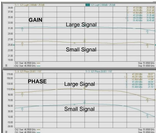
**Figure 6.** V-band linearizer custom frequency response.
