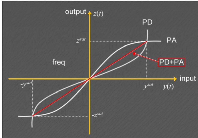
**Figure 1.** PD linearizer generates the opposite of a HPA's response in magnitude and phase.
