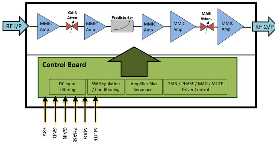
**Figure 5.** V-band linearizer functional block diagram.
