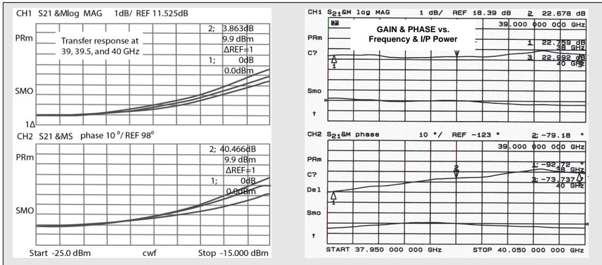
**Figure 14.** Linearizer transfer curve and frequency response to compensate a TWT, 38 to 40 GHz.
