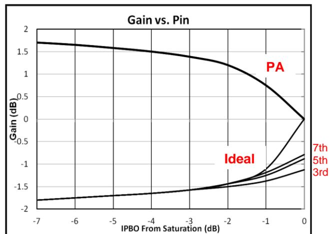
**Figure 2.** Gain vs. input power of cubic (3rd order) HPA with 3rd, 5th, 7th & infinite order PDL.
