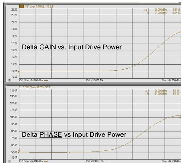
**Figure 7.** Linearizer transfer response (AM/AM, AM/PM).
