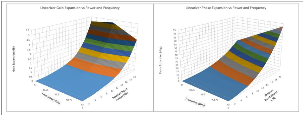
**Figure 3.** APDL surface for gain and phase compensation versus frequency.
