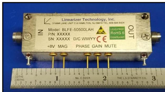
**Figure 4.** V-band linearizer module for a satellite uplink HPA.
