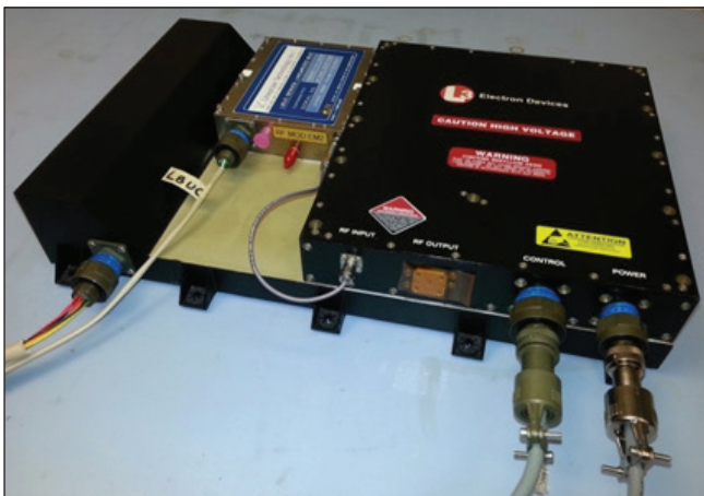
Figure 2: Complete X- to-Q-Band Transmitter (LMPM-T) with >50 W linear power is shown above. (Courtesy photo)
